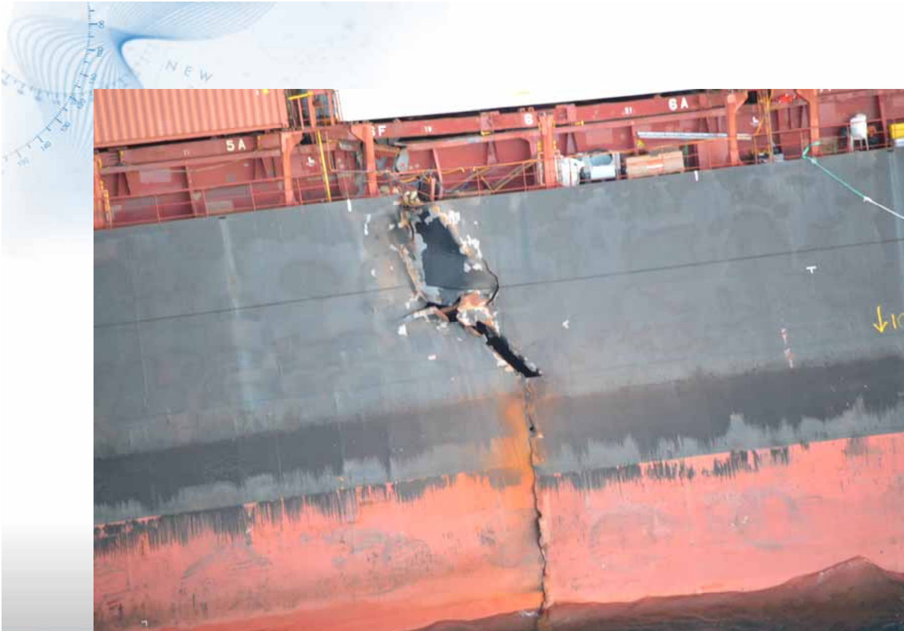
Rena – port side crack
